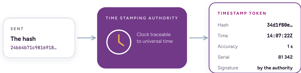
FIGURE 5 How a timestamp is obtained. The authority receives only the hash, never the document, and returns a signed structure with the time from its clock.
